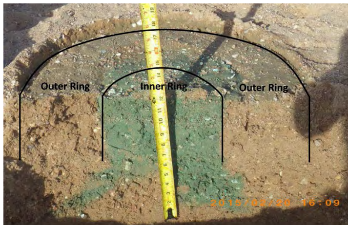
Fig. 5. Dye added to the inner ring of a double ring infiltrometer reveals the extent and direction of flow after steel rings have been removed (scale one the tape measure in inches, 1 inch = 2.54 centimeters) (image by author).
